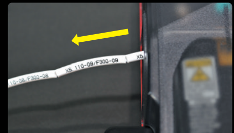
LETATWIN prints and half cut the tubing.
