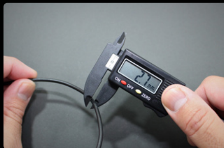
Check the outer wire diameter.
