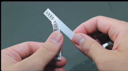
Stick printed tape onto Slide Plate
