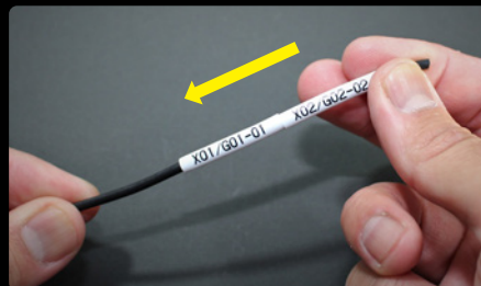
Insert 2pcs of the marked blocks
